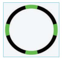
Any pipework carrying rainwater, to other points of use, that is located outside the building should be black plastic pipe marked with green horizontal stripes at the four quadrants as illustrated. (Available to purchase from FloPlast)
