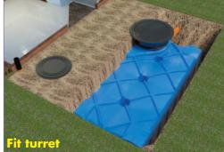
Top soil, clay, loam and other types of cohesive soils and materials with sharp edges are not suitable filling materials. Carefully backfill type 1 aggregate to all sides and up to at least 100mm above the top of the tank, compacting at every 100mm interval. It is also important to compact the material down into the column supports in the tank.
