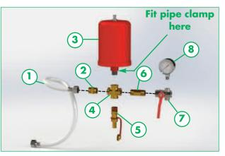
Connect the single length of the suction hose to the control panel unit. as shown, using the fittings provided. It is essential that this is water tight as any leaks will allow air into the system, resulting in pump failure and from this other potential problems can occur.
