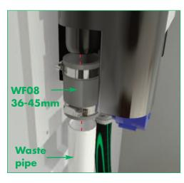
Using a WF08 36-45mm (not supplied) fitting connect a 43mm waste pipe (not supplied) to the overflow of the mainswater tank as shown. Run the waste pipe to a nearby drain, this will prevent water spilling onto the floor should the system overflow. The fitting and waste pipe are available from www.floplast.co.uk
