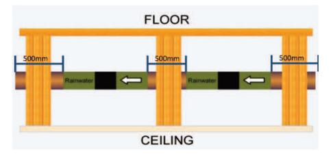
Marking of pipework in areas not easily exposed. When only small sections of pipework are visible for example between floor joists, a label should be applied at least in every void as demonstrated.
