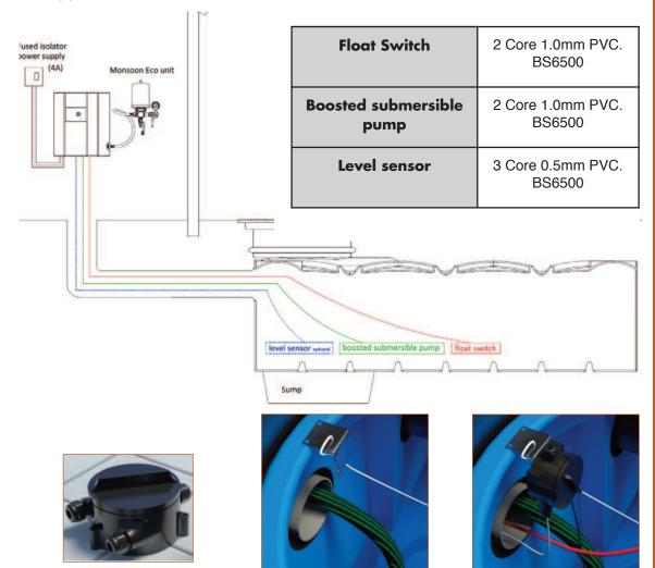
In cases where the cables are not long enough to reach the panel, run the cable into a waterproof junction box which needs to be mounted on the bracket in the turret as shown. Within the junction box connect it to a length of the specified cable and run that through the duct to the panel.
