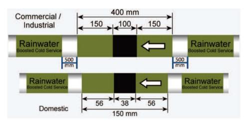
Examples of recommended labelling for pipework inside buildings. All pipework inside buildings should be labelled as shown above to ensure it is easily identifiable as a rainwater supply.
