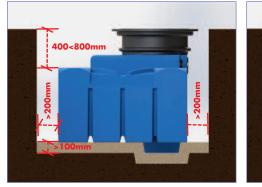
Carefully lower the tank into the excavation. Install and connect up all pipework, including the service duct for the floating suction hose and cabling.
