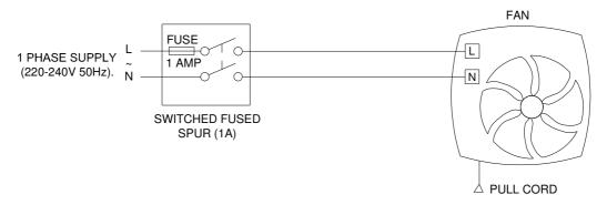
Fig. 4: VA100XT/VA100LT/VA100XHT (VA100LH & VA100XH LS CAN BE USED AS OVERRIDE)
