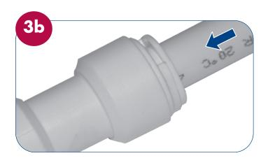
Insert the pipe into the fitting ensuring it passes through the o-ring until it reaches the stop point.
