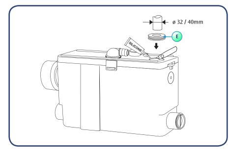
The washbasin can be connected in two ways. It can be connected to one of the side inlets (**see section 8**).
