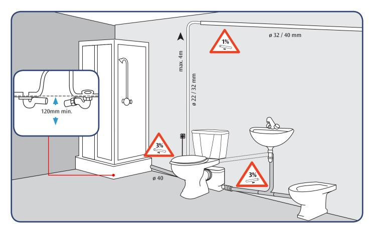
This unit must be connected to WC pan with a horizontal outlet spigot. The unit should be accessible for possible service. The unit should be installed by a qualified person.
