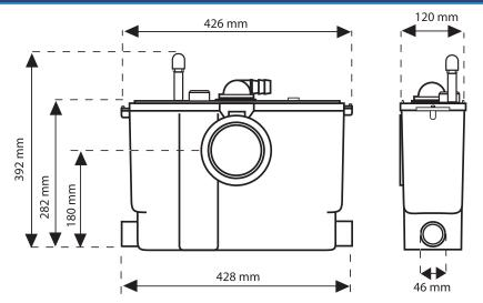
This pump/macerator has been designed to pump away the waste from a WC and the sanitary appliances in section 1.
