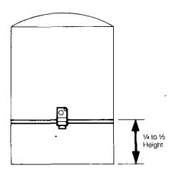
The cylinder thermostat should be mounted  $\frac{1}{4}$  to  $\frac{1}{3}$  of the way from the bottom of the cylinder.
