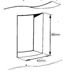
Remove a section of insulation as specified. Clean cylinder surface to ensure good surface contact.
