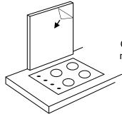
Once the glue or adhesive is fully cured or dried, you may now remove the protective plastic coating.
