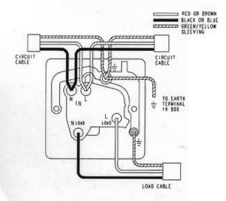
Unscrew cover and ease brown and blue wires from beneath strain relief bars. Remove knockouts in base and smooth any rough edges. Pass base over cables and screw it securely to the ceiling.
