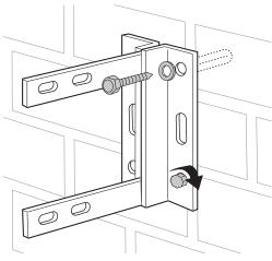
Fix the aerial to the wall fixing bracket using the 'V' bolts and nuts B.). Tighten firmly to secure.
