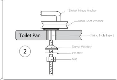
Insert the swivel hinge into the seat fixing hole at the rear of the ring/lid as shown in diagram above (Stage 1). Bolt the seat to the pan using the fixings in the configuration shown in diagram above (stage 2). To adjust the seat position to align with the pan see adjustment below. Once seat is in desired position fully tighten the nut using the fixing key supplied.
