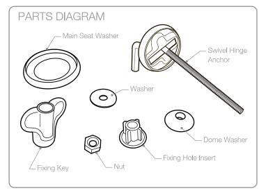
The seat is supplied with the above fixing kit (2x of each component except Fixing Key))
