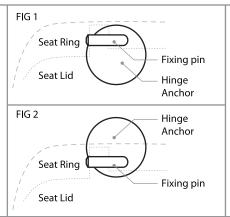
For minimum seat projection fit the hinge anchors as shown in Fig. 1.
