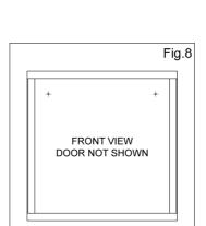
8. Hold the cabinet against the wall in its desired location and check that it is straight and level. Open the door(s) and mark the wall using the holes in the back of the cabinet as a guide. Drill 40mm deep holes in marked positions using a 6mm masonry drill and insert wall plugs. Align the holes in the back of the cabinet with the wall plugs. Insert the screws through the washers and holes in the back of the cabinet and screw in position.
