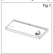
1. Mount the magnetic door catch onto the top panel. Use all four magnetic catch screws. Door catch must be fitted to opposite side of door hinge. (The magnetic door plate must be secured to the back face of the mirrored door to ensure that the catch works correctly)
