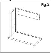
3. Place two wooden dowels into each end of the strengthening baton. Align the dowels and locate into side panel. (Wooden dowels must be glued into position.)
