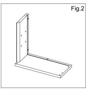
2. Secure side panel to base panel using two fixing screws. (Screws mounted from underside of base. To improve strength place small amount of glue on underside of side panel before securing into position.)
