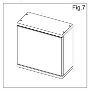
7. Place top panel onto cabinet carcase ensuring all screw holes, recesses, hinge grommets and dowels are accurately aligned with assembled cabinet. Secure top panel to both side panels with the four remaining fixing screws. Important: Please allow the glue to dry prior to fitting the cabinet.
