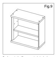
9. Insert shelf supports into hole recesses and ensure all supports are aligned accurately. Place the shelf in the cabinet and lower onto the shelf supports. (Door not shown)
