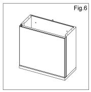
6. Place one of the door pivot pins into the hole recess situated on the base. (Hinge grommets need to be located in the recess of the top and base panels before inserting the pivot pin.) Locate mirrored door onto pivot pin and place the remaining pivot pin into the top of the door before securing the top panel.
