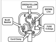
black. The brown wire must be connected to the terminal marked with an L or coloured red. The green/yellow wire must be connected to the earth terminal which is marked with an E or with the earth symbol. **WARNING:** Never connect live or neutral wires to the earth terminal of the plug.
