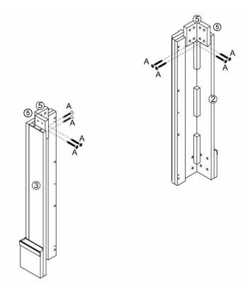
Screw the 4x connecting blocks (5) onto the rear of the left leg (2) and the right leg (3) with the 8x 25mm screws (A) provided.
