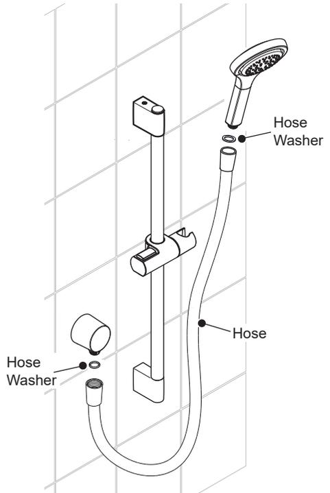
**Important! Flush the pipework before fitting the handset.**
