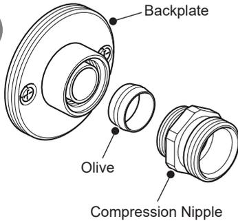
Fit the olive and compression nipple over the outlet pipe and tighten the compression nipple to  $25 \pm 1\text{Nm}$ .
