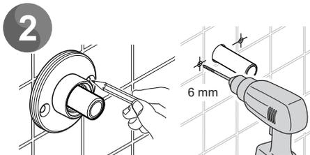
Mark the positions of the backplate fixing holes and remove the backplate.
