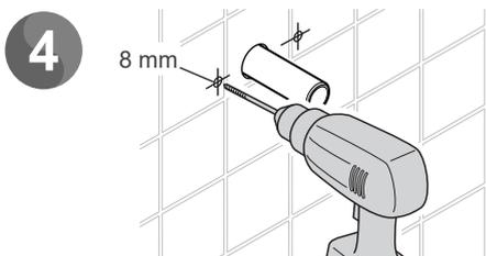
Drill the fixing holes and fit the wall plugs.
