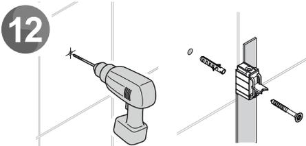
Drill into the marked holes to suit the wall fixings. Insert the wall plugs.
