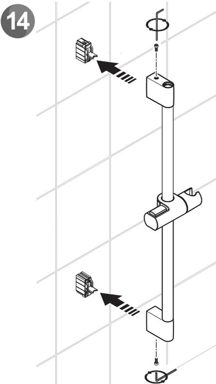
Position the slide bar assembly over the wall brackets and secure using the locking screws at both ends of slide bar. **DO NOT** overtighten.
