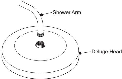
**Important! Flush the pipework before fitting the deluge overhead.**
