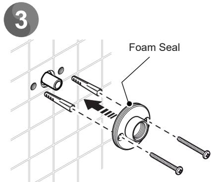
Carefully fit the backplate over the outlet pipe and secure with the fixing screws (supplied).
