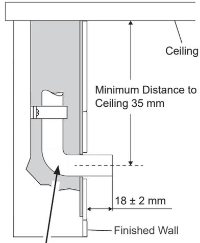
**Note:** 15 mm copper pipe must be used here.
