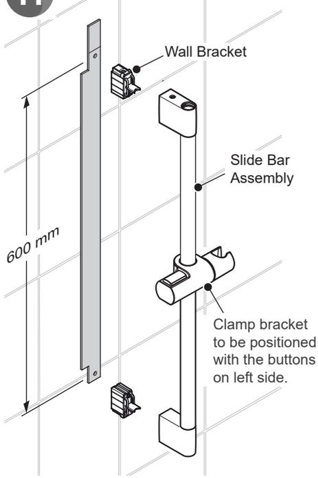
The slide bar should be fixed to the wall at a convenient height for all the users. It should be positioned so that water sprays down the centre of the bath, or away from the opening of a shower cubicle. Water should spray away from the Bluetooth® controller when the showerhead is held on the slide bar.
