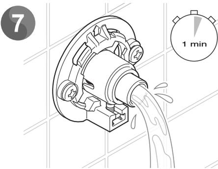
Flush pipework to clear all debris.
