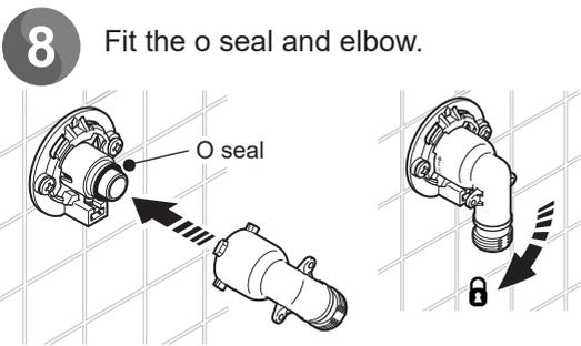
Fit the o seal and elbow.
