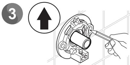
Disassemble the right angled connector assembly and mark the locations of the screw fixings.
