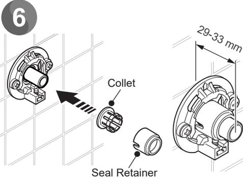
Fit the collet and seal retainer.
