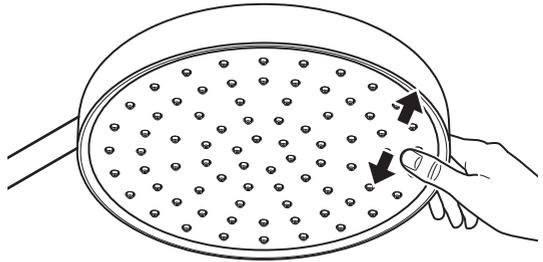
It is **IMPORTANT** to keep the Showerhead and Hose clean and free from blockage to make sure your shower performs to its optimum. The showerhead **MUST** be regularly cleaned and the hose **MUST** be regularly inspected to ensure there is no internal collapse or blockage that could reduce the flow.
