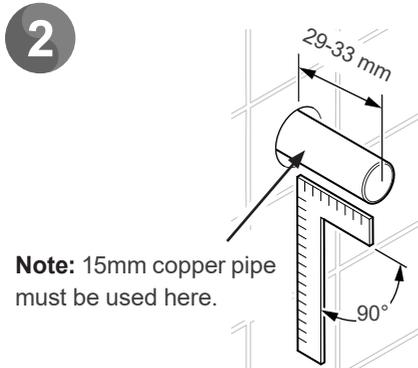
**Note:** 15mm copper pipe must be used here.
