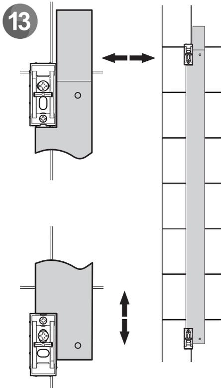
Use template to set correct distances between wall brackets. Fully tighten screws.
