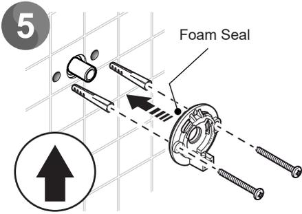
Secure the backplate to the wall so the foam seal is fully compressed.
