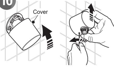
Fit the cover. Carefully lift the cover to locate the screw. Unscrew fully to lock using the 2.5 mm hex key supplied.
