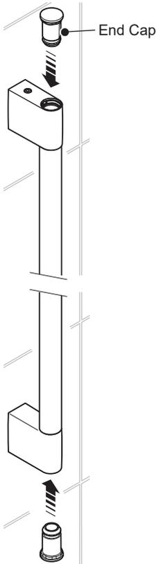
Fit the slide bar end caps into top and bottom of the slide bar assembly.
