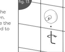
4. Unscrew and remove the Flexi-Fix bracket as shown. Be careful not to dislodge the auide that is now adhered to the wall.
