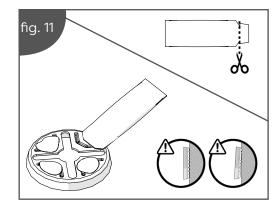
5. Open the sachet containing the adhesive and apply to the back of the Flexi-Fix bracket. (See Fig. 11)
