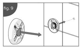
3. Peel off the adhesive sticker backing and press to wall on the marked center.
