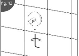
7. Install the Flexi-Fix Wall Mounted Accessory and tighten the grub screw to secure in place. Do not overtighten the grub
