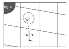
**3.** Install the Flexi-Fix Wall Mounted Accessory and tighten the grub screw to secure in place. **DO NOT** overtighten the grub screw.
