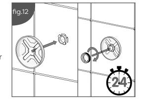
**6.** Re-install the Flexi-Fix bracket onto the guide and secure as shown.
