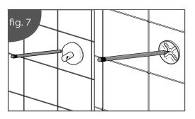
1. Place the Flexi-Fix bracket onto the wall and mark center for glueing. **DO NOT** attempt to install on grouting lines. (See Fig. 7)
