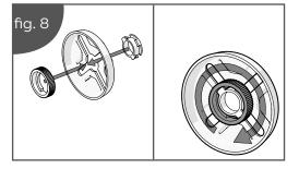
2. Assemble the Flexi-Fix bracket as shown.
