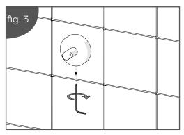
**3.** Install the Flexi-Fix Wall Mounted Accessory and tighten the grub screw to secure in place. **DO NOT** overtighten the grub screw. **(See Fig. 3)**
