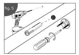
**2.** Drill holes and insert wall plugs. Ensuring the wall plugs sit flush with the wall.
