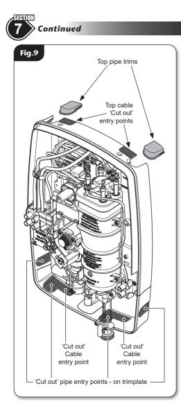
The backplate has removable top trims (top left and top right) that may be used for pipe entry and two additional sections (top left and top right) that may **ONLY** be used as a 'cut out' for top electrical cable entry **(fig.9)**.
