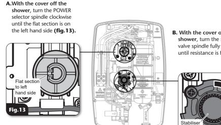
**B**. With the cover off the shower, turn the stabiliser valve spindle fully clockwise until resistance is felt (fig.14).
