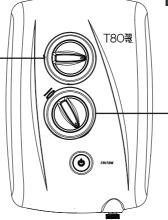
**D**. With the cover off the shower, turn the temperature control so that it goes to maximum HOT (fig.16).
