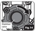
**C**. With the cover off the shower, turn the power selector to the COLD
