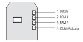
**REM 1** is for connection to a reception desk push button or a door intercom system. Pressing the button will cause the blue light to flash on the lock and release the lock for the pre-set time.
