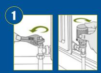
Close off both your radiator valves. (Although not necessary, we do recommenced this)
