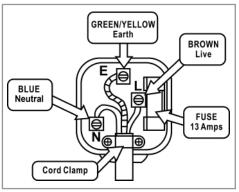
black. The brown wire must be connected to the terminal marked with an L or coloured red. The green/yellow wire must be connected to the earth terminal which is marked with an E or with the earth symbol. **WARNING:** Never connect live or neutral wires to the earth terminal of the plug.
