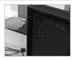
**Step 3:** Remove the outer spacer frame.
