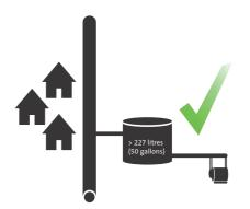
Fig. 2 Connection to mains via storage tank
