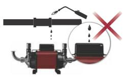
Fig. 9 Solder flux causes damage to plastic parts
