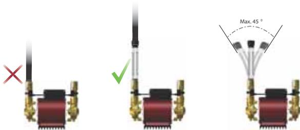
Fig. 18 Connecting the flexible hoses
