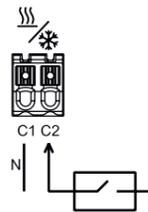
**Note:** when several (max 3) controllers are used only one heating/cooling input is required. The complete system will change to cooling mode.
