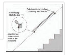
Drill ø8mm diameter holes for the wall plugs being used, insert wall plugs and using screws provided, screw the Connecting Wall Bracket to the wall. Tighten the two tube retaining screws at either end holding the tube in place using the allen key provided, ensuring you do not over tighten.
