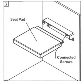
Fasten the PU seat pad onto the bracket and ensure the seat pad can be moved along the guide channel smoothly, then these screws can be locked.
