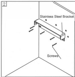
Fix the seat bracket to the wall by screwing into the mounting positions.
