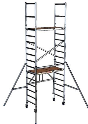
16 Reposition the 1<sup>st</sup> platform from its original position to the 1<sup>st</sup> rung of the folding frame.
