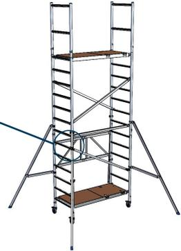
18 From the trapdoor position, fit two guardrails on the 15<sup>th</sup> rung (on both sides).
