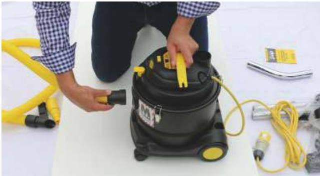
13 Push hose end into suction port
