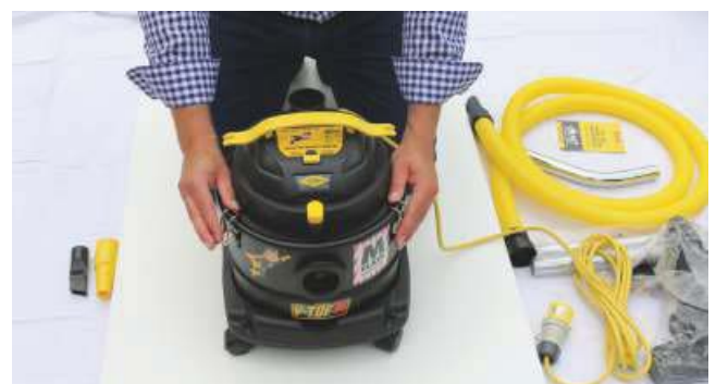
12 Refit head and ensure all three clamps are fastened
