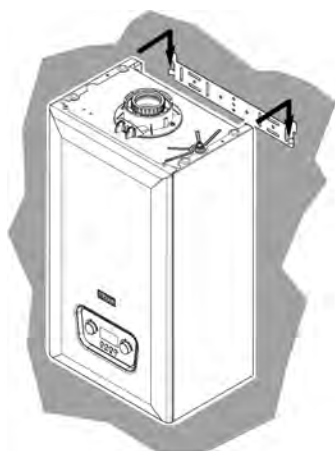
Fig.30 Mounting the boiler
