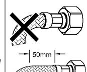
Both ends of the hose must have a minimum 50mm straight section before any bend.
