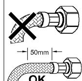
Both ends of the hose must have a minimum 50mm straight section before any bend.
