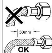
Both ends of the hose must have a minimum 50mm straight section before any bend.
