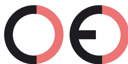
False CE Mark (too far)
