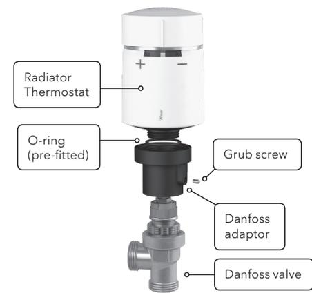
Slide the larger black plastic adaptor small end first over the valve. Make sure that the hole containing the grub screw is facing away from you. This way, once its mounted, the markings of the Radiator Thermostat will be in the required position. Use a 2mm size Allen key to tighten the grub screw. Now screw the Radiator Thermostat onto the larger black plastic adaptor until tight.
