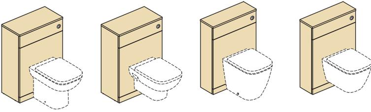
**IMPORTANT** - If installing unit with wall hung pan - replace bottom panel "Lift-on" clips with loose "Push-on" clips supplied
