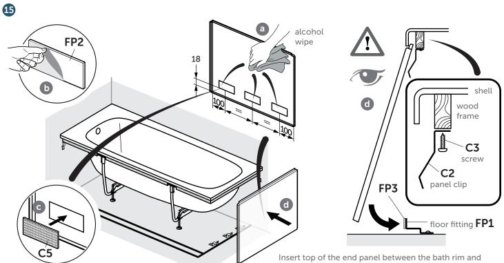
Insert top of the end panel between the bath rim and panel clips and push the bottom of the panel against the 'reattachable fastening' tape on the brackets.
