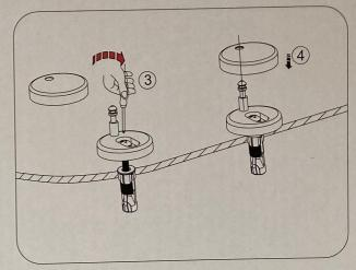
3 Tighten the screw using a screw driver but not firmly fixed. Determine the right position of the hinge pin by placing the seat on the pan and comparing the pins against the pin holes in the seat. Then, continue to tighten the screw until it is firmly fixed.
