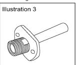
Step 3 - Screw the fixing bridge onto the wall plate using a 22mm a/f spanner. Flats have been produced on the wall plate to take a 47mm spanner (Illustration 3).
