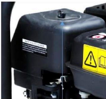
1. Air filter cover wing nut.
