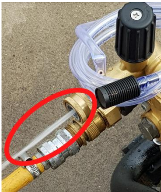
Fig3 pos.9: High pressure outlet : This is where the high-pressure hose connects.
