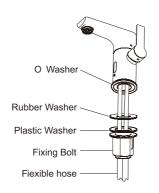
Step one: Take away the rubber washer, plastic washer and fixing bolt.
