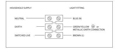
Check that..... You have correctly identified the house wires. The connections are tight. No loose strands have been left out of the connection block.
