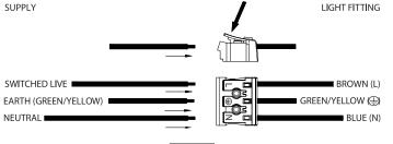
Loop \_\_\_\_ Loop Spare block supplied in fixing pack
