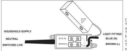
Check that..... You have correctly identified the house wires. The connections are tight. No loose strands have been left out of the connection block. The terminal block box cover is securely re-fitted.
