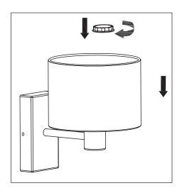
Fitting/Replacing the bulb - Max. 40W E14 Golf
