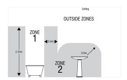
This product has no special protection against the ingress of moisture, and is rated as IP20. This product is not suitable for use in Zones 0, 1 or 2, of a bathroom. See diagram.
