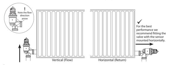
If you are not installing a Danfoss lockshield valve (supplied in sets code, 013G7662 & 013G7663) ensure that the lockshield is fully open. No balancing on the lockshield/return pipe.
