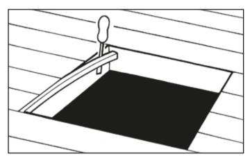
**I.4** Screw hinges (D5) to one edge of the trapdoor using 20mm (3/4") wood screws (D6).
