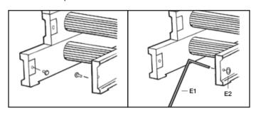
**4.4** Lower 'V' rod to the loft floor, in line with the centre of the ladder.
