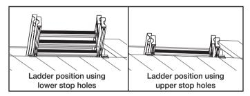
One Check the ladder angle against the safety label or refer back to Deployed Requirements on page 2.
