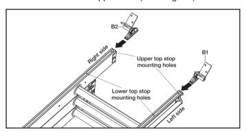
L2 Slide the hinge guides past both sets of top stop mounting holes, so that the hinge guides are below the top stops, when they are fitted in section 2.
