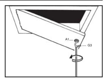
10.3 Locate the stowing hook/key (E3) over and at the centre of the REAR ladder section bottom rung and steadily pull the ladder outward and downward until both top stops reach and make contact with the hinge guides.
