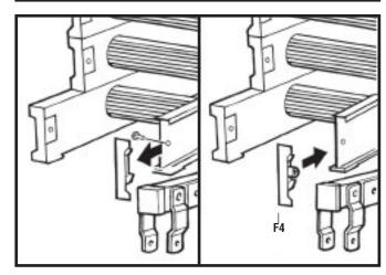
8.9 Locate the power arm linkage plates either side of pivot tip (F4)/ladder stile and align all holes.
