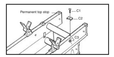
**5.3** Fix the additional top stops using two M4 bolts and nuts supplied (C1 & C3).
