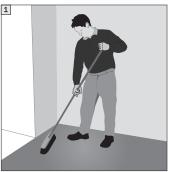
All construction dampness for example newly applied screed must be completely dried out before installation. The surface should be clean, flat, level (<3 mm over 2 m area) and dry.</p>
