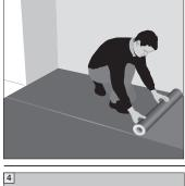
© Cut and lay using spray adhesive or staples to secure to the floor, All seams should be joined using underlay tape prior to the carpet being fitted.
