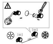
hot inlet on left, cold inlet on right
