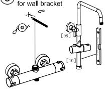
using the plugs and screws supplied to mount the wall bracket
