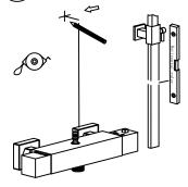
6 using the plugs and screws supplied to mount the wall bracket
