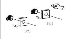
mount the mixer, before connecting the mixer, water must be flused through the pipes to remove any debris
