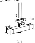
fix the riser pole to the mixer, then fix the riser pole to the wall bracket
