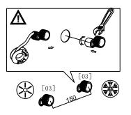
hot inlet on left,cold inlet on right
