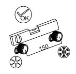
3 screw coverplate over the offset connectors
