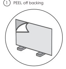
Make sure all corners are well protected from any hard surfaces. Carefully peel off the protective film back. Take care not to remove the self-adhesive backing.
