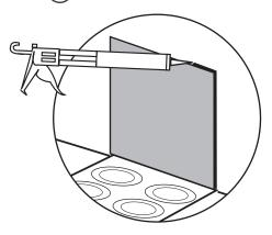
Use the Clear Silicone Sealant to seal around all four sides of the splashback. Take care to ensure that the sealant is no more than 2.5mm in thickness.
