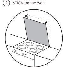
Place the bottom edge of the splashback to the rear of the hob, cooker, range or sink. Push it to the wall and apply firm even pressure with a cloth.
